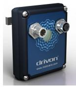
This optional module enables the communication through standard Profibus DPV1 field bus. This module makes it possible to assign a network address through on-board manual rotary selector switches. In addition, the user can activate a termination resistor through jumpers as required. Two M12 B-code connectors (a male and female connector) are provided on the outside of the module for Line connection to field network.
