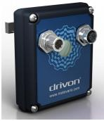
This optional module implements hardware and software interfaces for Real-Time-Ethernet networks over Ethernet IP profile. Two M12 D-code a female connectors are provided on the outside of the module for Line connection to field network.
