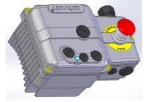
This option consists in an external emergency stop button that activates the Drivon's STO function. Pressing the button cuts power to the motor in full safety in accordance with EN ISO 13849-1 and EN61508, whereas the inverter remains powered.
